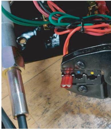
6. Install newly crimped connectors onto the toggle switch tabs (as shown). Make sure they are fully engaged.
