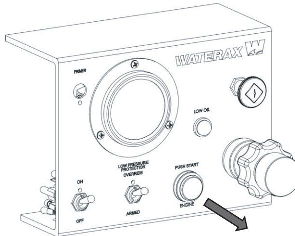
2. Install the new toggle switch as shown.
